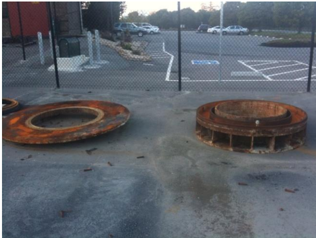
Original base & turntable, Biotower No. 2
